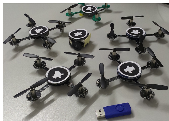
(e) Swarm of robots tagged with WhyCode markers
