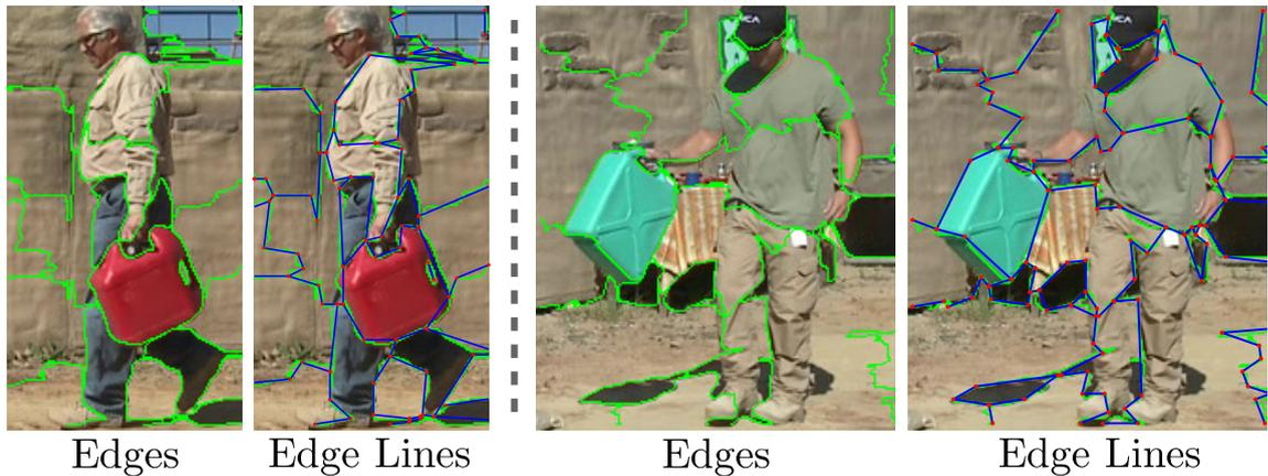
Figure 3.3: Two examples of obtaining edge lines from edges. In each case the left image shows the edges obtained by using the Quick Shift algorithm in green. The right image shows edge lines in blue where a red dot is the start or end of the edge line.
