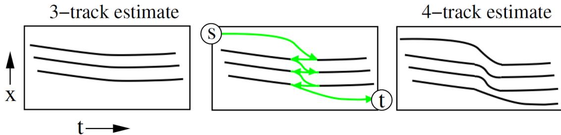
Figure 2.10: Tracking process of Pirsiavash et al. [63] where they derive an optimal interpretation of a video with  $k + 1$  tracks by locally modifying the solution of  $k$  tracks. In this example they use a 3-track estimate and obtain a 4-track estimate by using a shortest-path computation that pushes the flow from a source (s) to a terminal (t).
