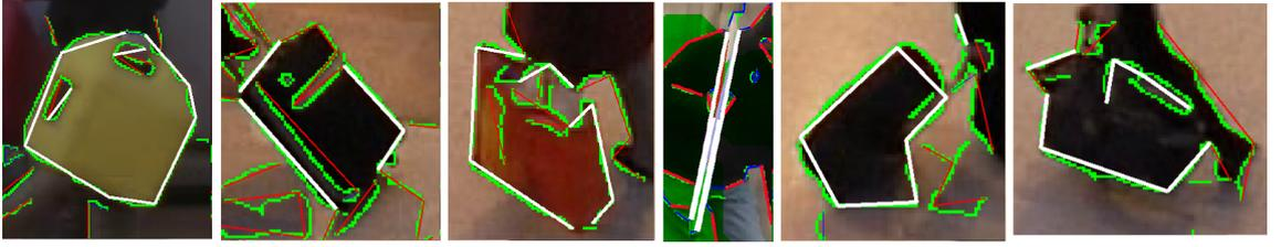
Figure 3.8: Examples of using geometric shape models for carried object detection. Green segments represent edges from the Canny edge detector and the white chain lines represent the convex/elongated objects found in the level-wise mining procedure.
