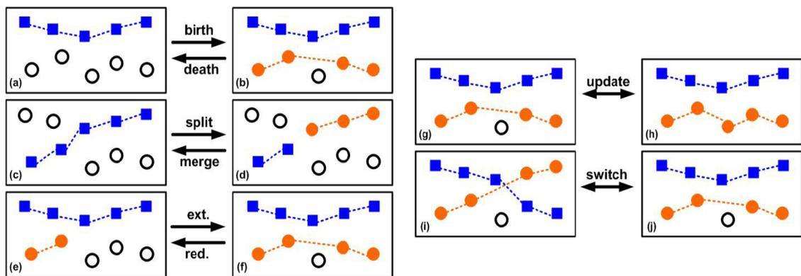
Figure 2.13: The set of moves applied in the Markov chain Monte Carlo data association tracker by Oh et al. [59] to create or modify track partitions of observations.
