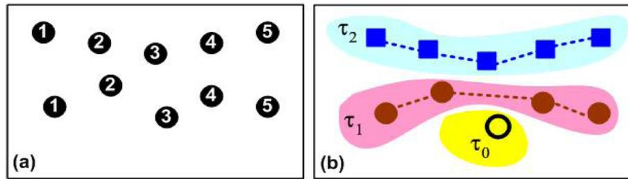
Figure 2.12: The tracking process of partitioning observations in image (a) into tracks in image (b) [59]. The number in each observation node represent its frame number.
