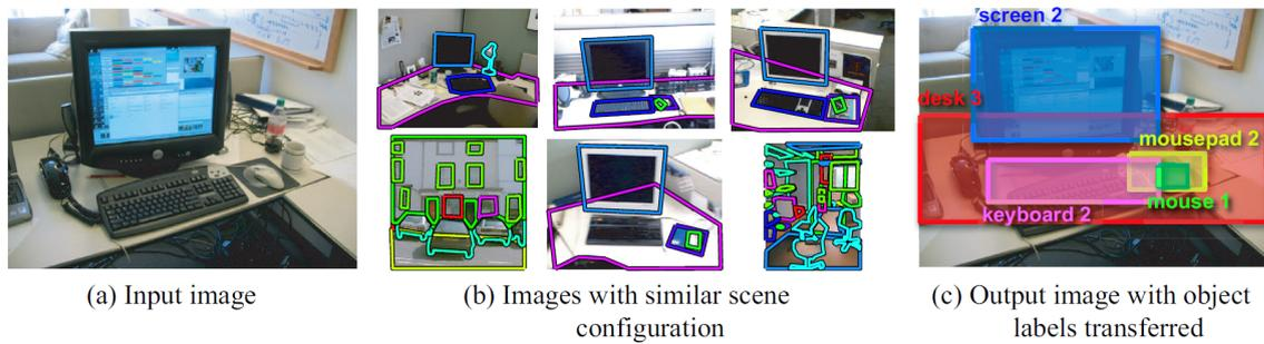
Figure 2.16: The approach of Russell et al. [69] for *gist* based contextual object recognition of a target image (a). Using scene *gist* they match the target image to other images that have a similar *gist* (b). They then use the labels in the best matching images and transfer them onto the target image.
