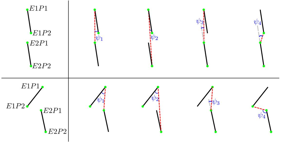
Figure 3.9: The four different angles  $\psi$  used to obtain a co-linearity measure between two edge lines  $E1$  and  $E2$ . Each edge line has a start point  $P1$  and an end point  $P2$ . Red lines are used to connect two green edge point to each other. An angle  $\psi$  is obtained between the red edge line and a black edge line between two green points.
