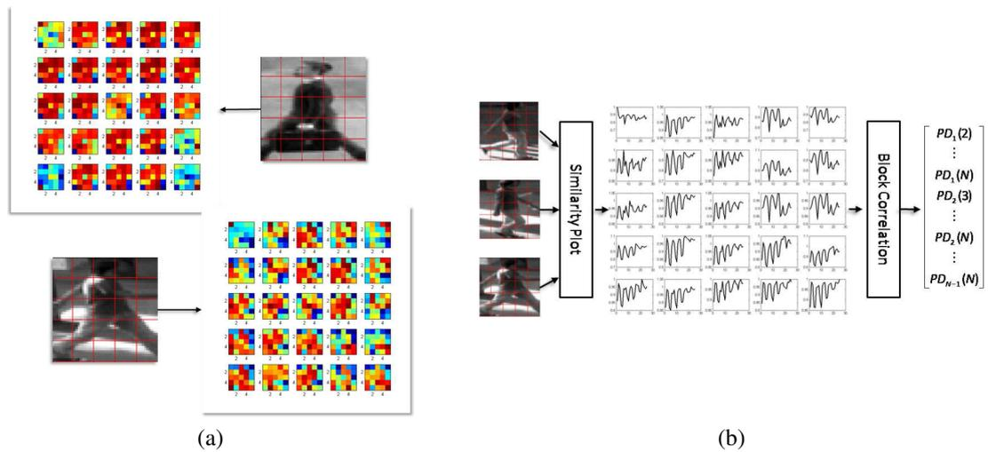
Figure 2.7: The use of periodicity dependency by Senst et al. [71] for carried object detection.
