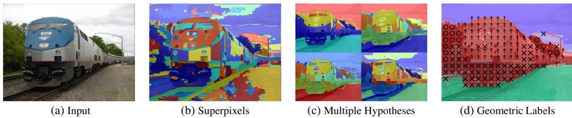
Figure 2.17: Geometric context labels proposed by Hoiem et al. [40]. For an input image (a) they obtain superpixels (b) in which they obtain curious groupings for (c). In (d) they then assign one of three labels to each image pixel, (i) being part of the ground plane, (ii) belonging to a surface that sticks up from the ground or (iii) being part of the sky.
