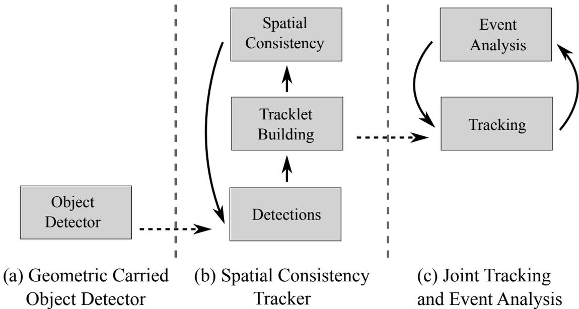
Figure 1.2: The three main frameworks of this thesis namely (a) Geometric Carried Object Detector (b) Spatial Consistency Tracker and (c) Joint Tracking and Event Analysis. Dotted arrows represent the link between the output of one framework to the input of another. The solid arrows represent internal links between elements within a framework and the notion of influence between them.
