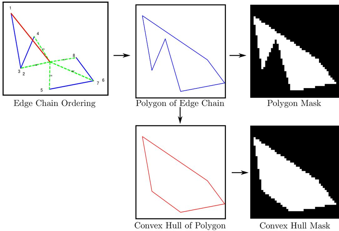
Figure 3.7: Example of an ordered set of edge line, the corresponding polygon leading to an object mask with a non convex shape and the convex hull of the polygon.
