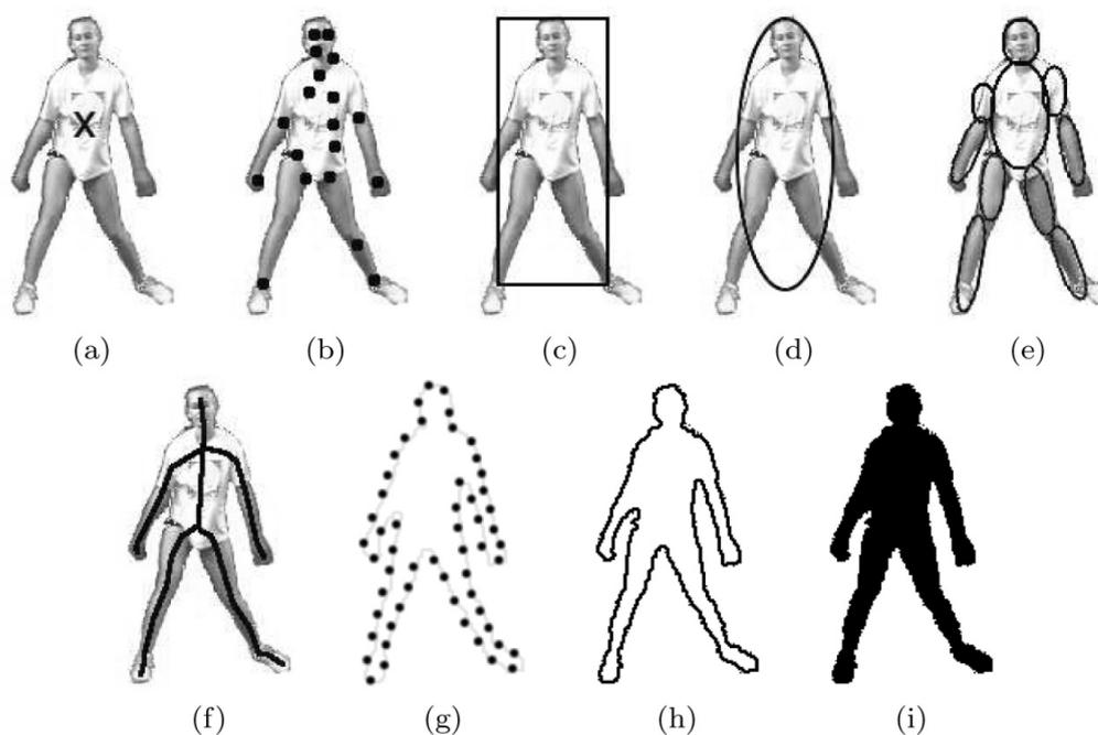
Figure 2.9: Object representations categorised by Yilmaz et al. [101]. (a) Centroid, (b) multiple points, (c) rectangular patch, (d) elliptical patch, (e) part-based multiple patches, (f) object skeleton, (g) complete object contour, (h) control points on object contour and (i) object silhouette.
