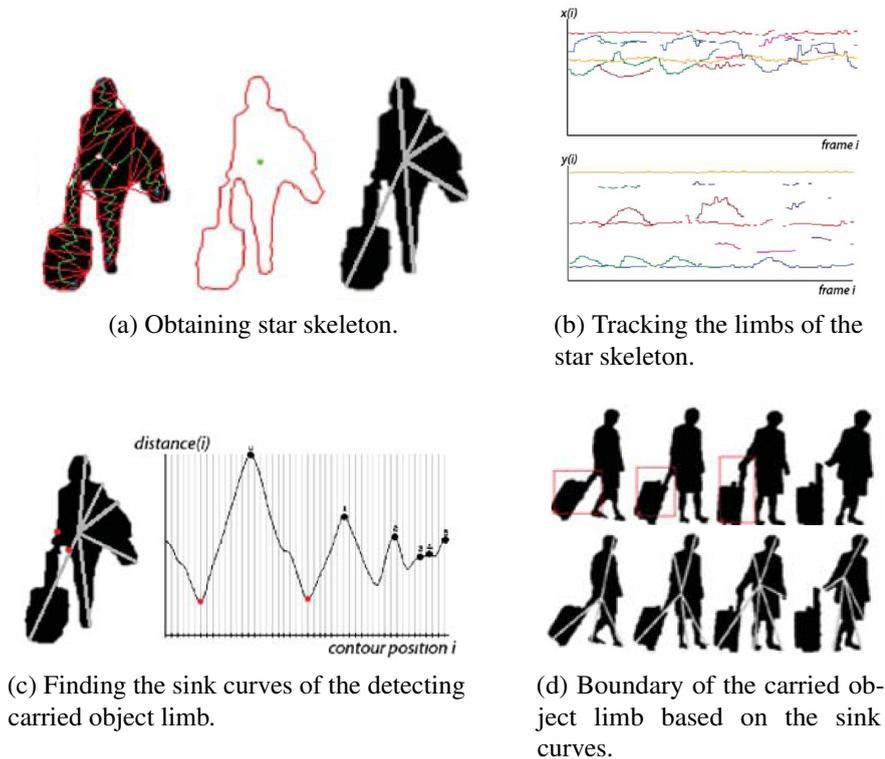
Figure 2.4: Chayanurak et al. [16] carried object detection using star skeleton.
