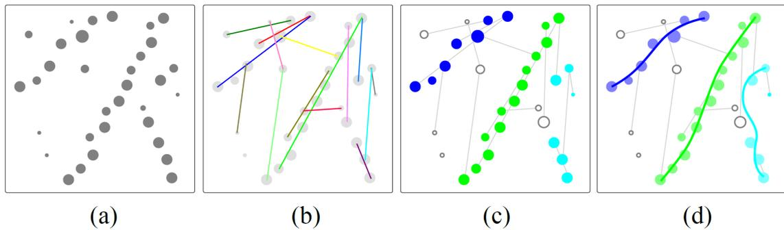
Figure 2.14: The discrete-continuous tracking process of Andriyenko et al. [4]. Given a set of unlabelled object detections in (a) and a set of possible trajectory hypotheses in (b) this tracking process assigns labels for all detections, presented in (c), and re-estimates the trajectories, presented in (d). This process alternates between discrete and continuous tracking where they are performed jointly using an energy minimisation approach.
