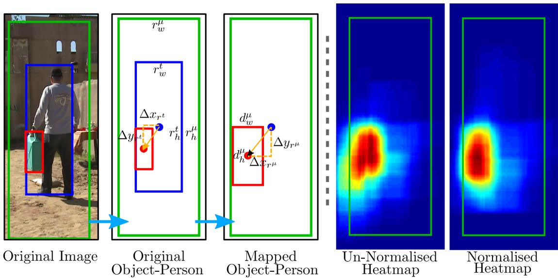
Figure 4.3: The process of mapping a person bounding box to a normalised person bounding box. The mapping is also applied to the object to preserve the object-person relationship. By comparing the normalised heatmap to the un-normalised heatmap, we can observe that the normalisation process greatly enhances the relative consistency as the normalised heatmap obtains a more localised distribution representing the true location of the object.
