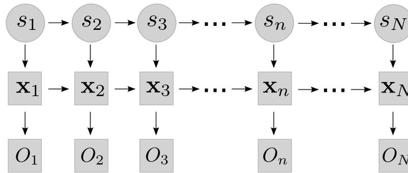
Figure 7.1: A proposed switched Kalman filter architecture which would perform both tracking and event analysis under one architecture. The bottom layer is for detection observations, the middle layer represents the layer and the top layer represents the events where  $N$  is the total number of frames.
