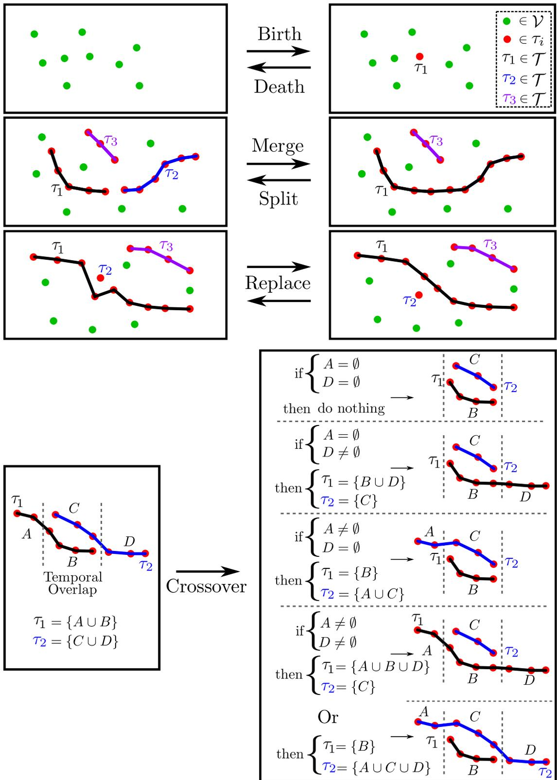
Figure 4.6: Examples of moves used in the SCT optimisation procedure. Each row showcases the affect of a move being applied to a set of unused detections in  $\mathcal{V}_{\mathcal{T}}$  and a set of tracklets in  $\mathcal{T}$ .
