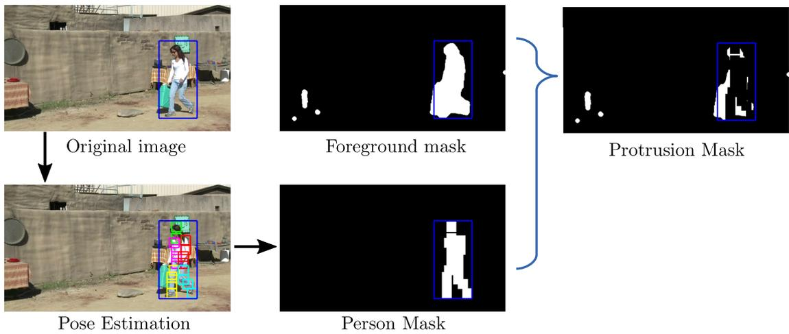
Figure 3.2: Process of obtaining the protrusion mask.
