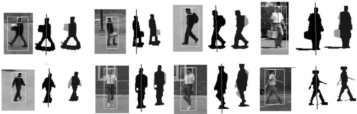
Figure 2.1: Backpack [37]: Examples of symmetry based segmentation of potential carried objects with initial detected head location, computed symmetry axis and final non-symmetric region segmentation. Combined with periodicity analysis these regions may be considered as carried object regions.
