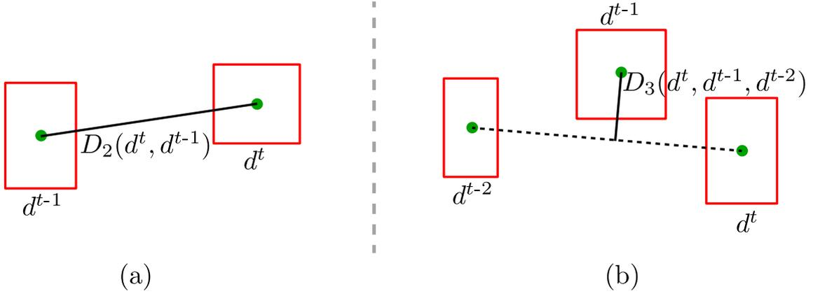
Figure 4.4: Examples of distance functions  $D_2$  and  $D_3$  used as part of the tracklet suitability measures. The distance is the length of the solid black line, obtained based on the centre points of detection  $d$ .
