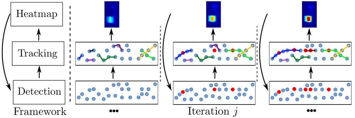
Figure 4.5: The architecture of our framework and examples of iterations in the optimisation process of our spatial consistency tracker as a result of applying the aforementioned framework. The cyclic nature between tracking and the heatmap emerges as more tracklets are built in the tracking stage resulting in a more accurate heatmap over more iterations, which in turn promotes more detections (red) for the tracking process.
