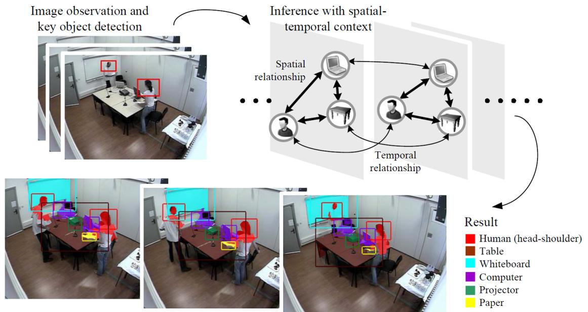
Figure 2.18: Object recognition and tracking using spatio-temporal context by Li et al. [53]
