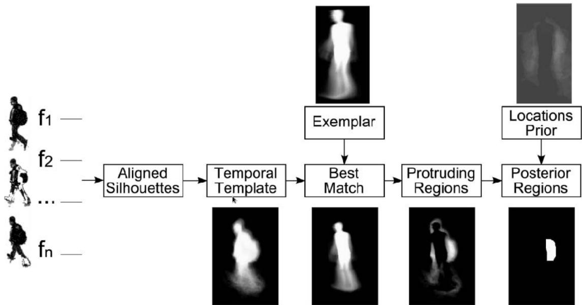
Figure 2.2: The pipeline of segmenting the carried object region in Damen and Hogg [24]. By comparing the temporal template of a person with a best matched exemplar template, protrusion regions are found which lead to carried object detections.
