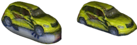
Fig. 8. Reconstructed polygon mesh before and after cropping using the convex hull of the reconstructed point cloud.
