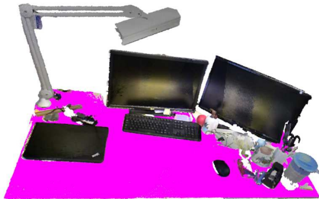
Fig. 1: An example point cloud with a desktop scene. All the points detected by the PPR technique as desktop surface inliers are highlighted in pink, outliers have their original color. Notice how the object points are avoided from being misclassified as inliers. The typical result from plane extraction without our refinement on this scene is to include the bottom few centimetres of objects as table points.
