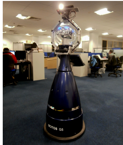
Fig. 3. Our Scitos G5 robot – equipped with two RGB-D sensors and a laser scanner – in our open office environment.
