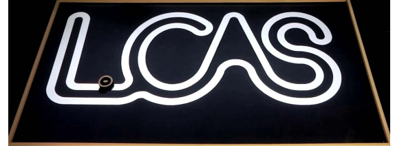
Fig. 5. Localization precision experiment: A snapshot of the experiment with Colias-Φ robot following a complex path. (LCAS stands for the Lincoln Centre of Autonomous Systems)
