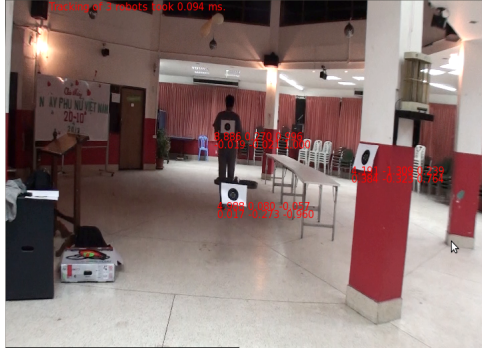
Fig. 6 Markers on the target and AR.Drone localizing their world-coordinate position with reference to an additional calibrated camera.
