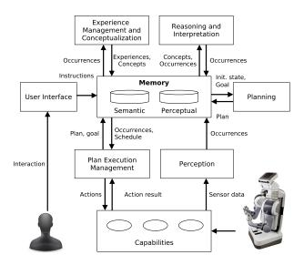
Figure 1: High level overview of the RACE architecture.
